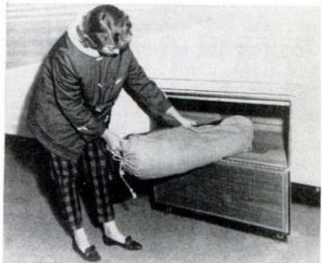
OUTSIDE BINS allow heat to escape. Insulate interior surfaces with foam or fiberglass and pack a quality sleeping bag for personal warmth on cold nights
